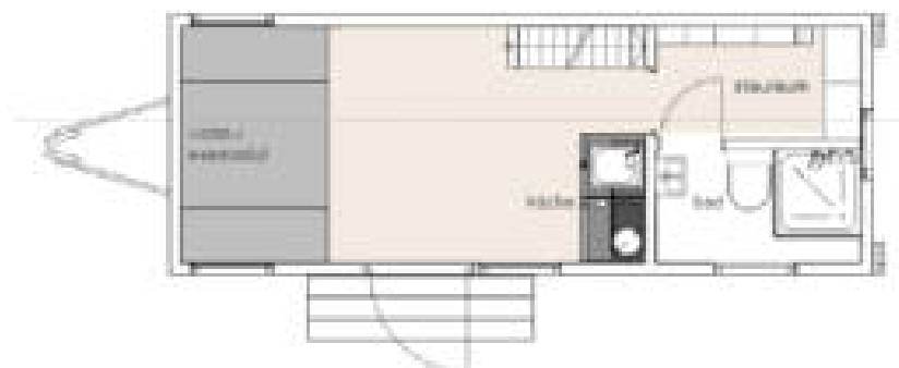
Abbildung 3: Grundriss Tiny House Modell "Living House" 36
